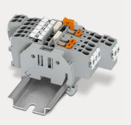
The TOPJOB® S Disconnect and Test Terminal Blocks allow you to quickly and safely disconnect circuits. The orange-colored knife disconnects or disconnect plugs are located between the conductors and provide visual confirmation of the switched status.
